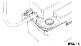
**Step 5:** Secure hose by pushing small clamp forward towards the pump. (Fig. 15)
